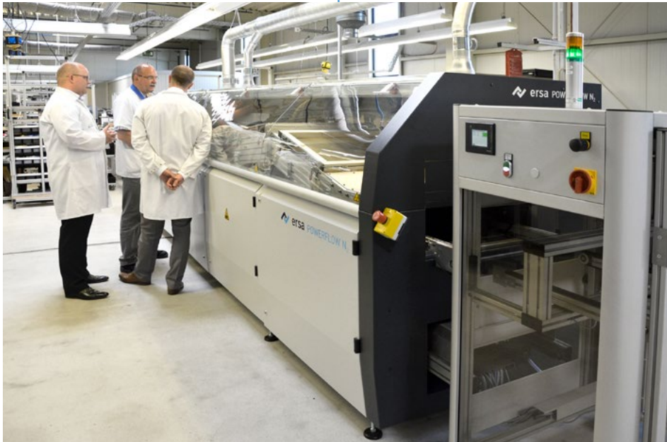
The through-hole line with the Ersa POWERFLOW N 2 full tunnel wave soldering system in the STG-BEIKIRCH production.
