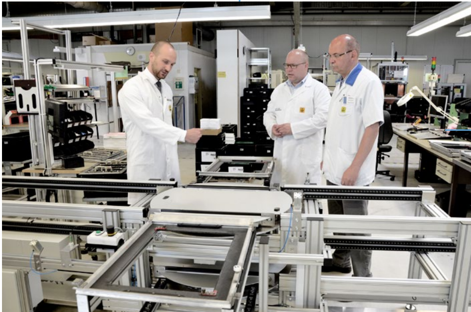
In its electronic manufacturing, STG-BEIKIRCH relies on the RFID technology, which allows for traceability, solder program selection and return of the pallet to the corresponding workstation.
