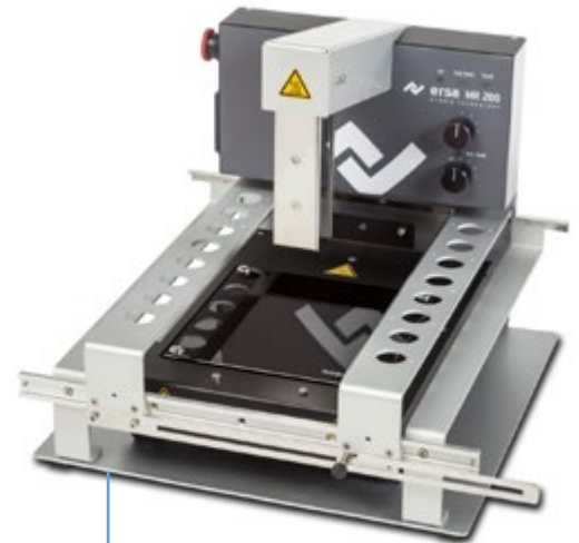
„Out-of-the-Box“ – Compact Ersa Hybrid-Rework-System HR 200
