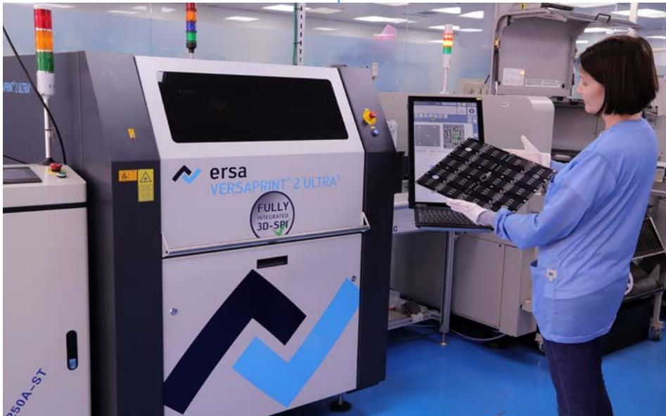
*VERSAPRINT 2 with operator inspecting a printed circuit board.*
